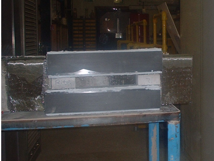
Plate 1. CFRP plate concrete specimens, where the artificial blisters are embedded between the interface of composite and substrate
